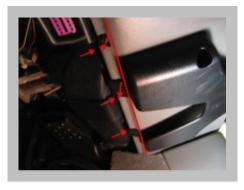
Now you need to remove the the dash button trim piece. To do this use a blunt butter knife and pry it off from the bottom. Be careful because it can take some force to remove. Now that the cover is off, remove the dummy plug and insert the wiper dial into the trim piece.
